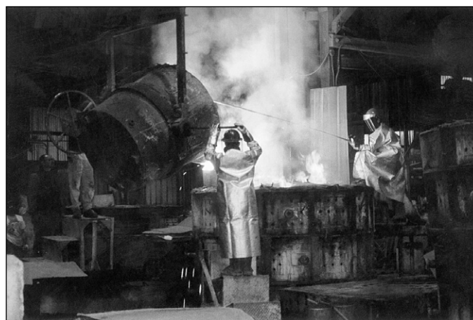
Figure 16.6: Foundry workers performing metal pour into a sand-filled form for steel manufacture. The worker on the left is controlling the rate of the pour by controlling the angle of dip of the crucible. The worker on the right uses the long pole with bar to prevent floating slag (waste products generated during the melting process) from getting into the form. There are several unsatisfactory safety practices that are occurring simultaneously during this pour, which include the absence of respiratory and hearing protection, face and body shielding, or proper elevation equipment for all workers present. Courtesy of Susan Swan.
