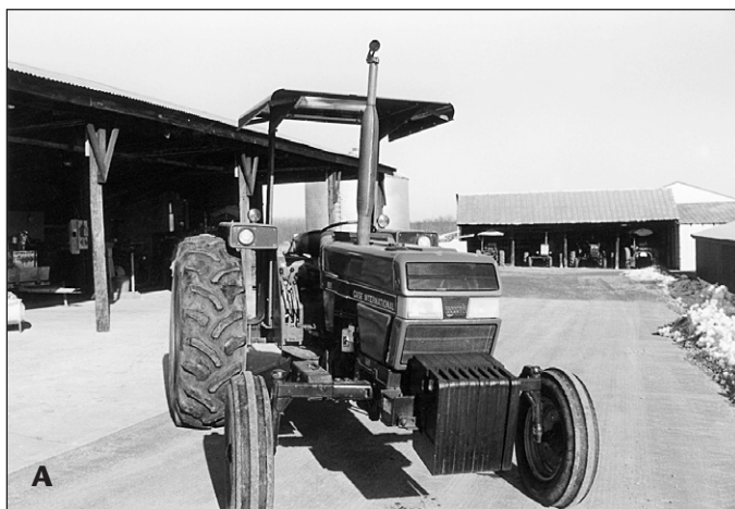
Figure 12.5: (a) and (b) Modern tractors with rollover protection system (ROPS). Note the tractors have a wide front end and front-end weights to counterbalance any equipment attached to the drawbar at the rear.
